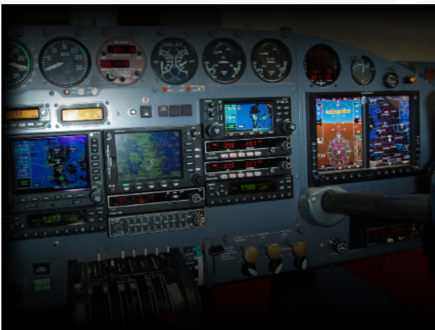
Garmin G600 Installation in Cessna 414 by SA.
