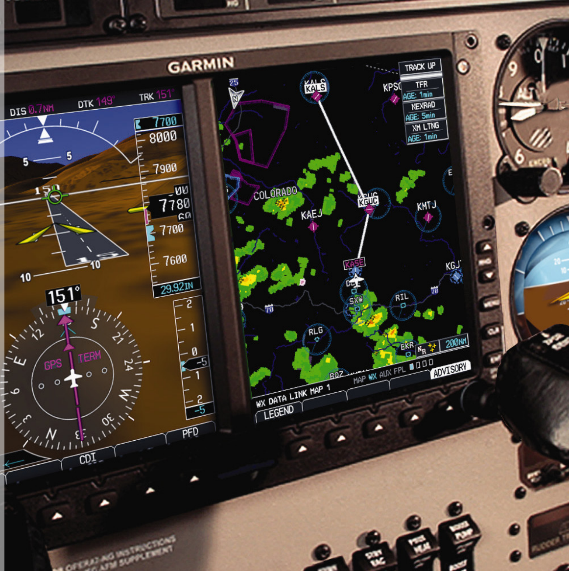
Garmin G500/G600 Multifunction- & Primary Flight Display
