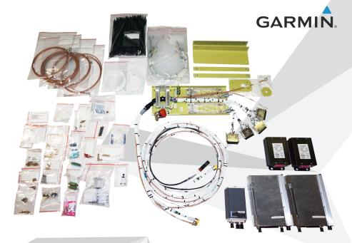
All new units are accommodated on a shelf, wired on the bench and installed in the avionics rack RH. The equipment on the shelf are being connected to the aircraft systems through two pigtail connections. Two new break connectors are installed on a bracket, and the break connector bracket are installed on the existing 28VE rack.
